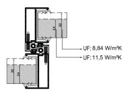
CAM KALINLIKLARI (GLASS THICKNESS) : min.24mm - max.32mm
