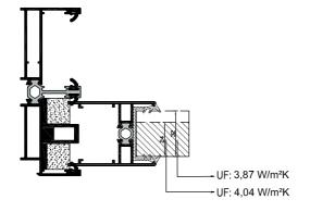
CAM KALINLIKLARI (GLASS THICKNESS): min.24mm - max.32mm
